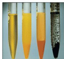
(NH<sub>4</sub>)<sub>2</sub>S CdS Sb<sub>2</sub>S<sub>3</sub> PbS
